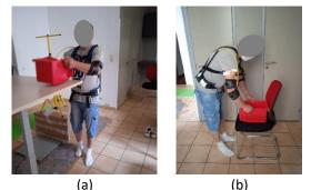
(a) (b) Figure 3: dynamic task: 6 kg load to carry (a) from a table (b) to a seat 3 m away
