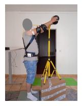
Figure 1: static task with arms at 105°, 1 kg per hand
