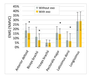
Figure 8: Mean EMG values normalized by the MVC for each muscle, with and without the exoskeleton. Asterisks denote significant differences (p < .05) from the reference condition (without exoskeleton)
