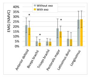
Figure 6: Mean EMG values normalized by the MVC for each muscle, with and without the exoskeleton. Asterisks denote significant differences (p < .05) from the reference condition (without exoskeleton)
