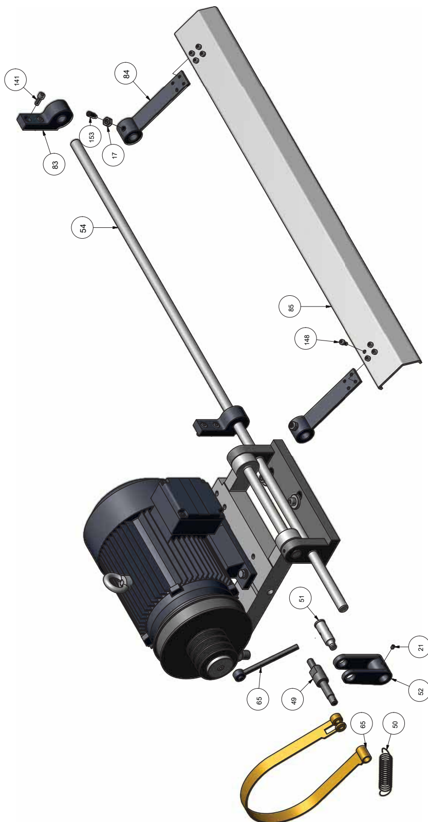
8-24: Spindelbremse - ruptura husillo
