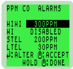
Fig. 3-10 Carbon Monoxide Alarms
