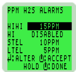
Fig. 3-11 Hydrogen Sulphide Alarms
