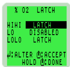
Fig. 3-14 Oxygen 'LATCHING' Alarm Option
