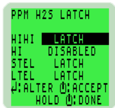
Fig. 3-16 Hydrogen Sulphide 'LATCHING' Alarm Option
