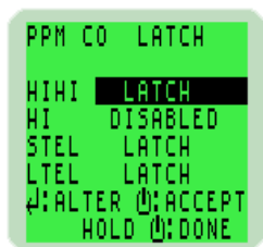
Fig. 3-15 Carbon Monoxide 'LATCHING' Alarm Option
